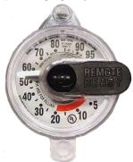
and the other is a pressure gauge that will say "PSI" somewhere on the dial. The level of the tank will change with temperature. In cold weather, the tank level will read lower than it will during warm weather, even though it has the same number of gallons in the tank. Customers may perceive they have a leak if they check the tank in the afternoon of one day, and then recheck the morning of the next day, as the tank levels may be different, depending on the temperature change.
